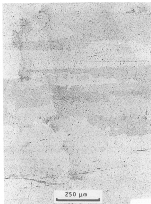
Figure 1 Optical micrograph showing the grain structure of wrought MA 754 alloy.
